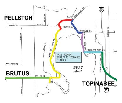
PHASE 1, CRUSHED LIMESTONE PATHWAY, COMPLETED 2014 PHASE 2, PAVED PATHWAY, COMPLETED 2020 PHASE 3, UNDER DEVELOPMENT, EXPECTED 2021 PHASE 4, COMPLETED ROAD SHOULDER, 2020 PHASE 5, COMPLETED ROAD SHOULDER 2017 FUTURE PLANNED CONNECTION TO NC STATE TRAIL FUTURE PLANNED CONNECTION TO NW STATE TRAIL
